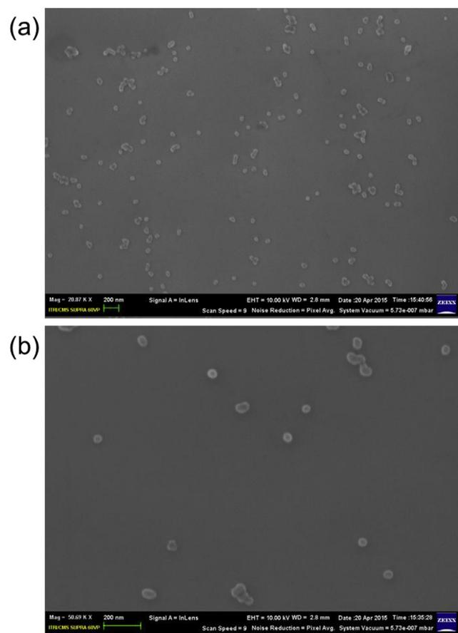
**Fig. 4** – SEM micrographs of FZO-50 nanoparticles deposited on bare Si chip at magnification of  $20 \text{ k}\times$  (a) and  $50 \text{ k}\times$  (b).
