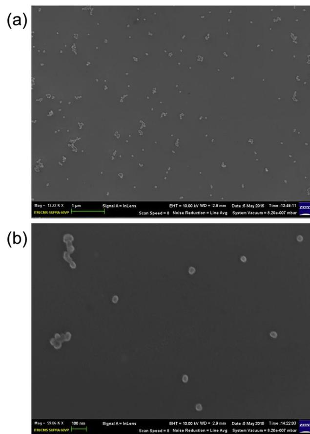
**Fig. 5** – SEM micrographs of ZnO-610 nanoparticles deposited on modified Si chip at magnification of  $13 \text{ k}\times$  (a) and  $60 \text{ k}\times$  (b).
