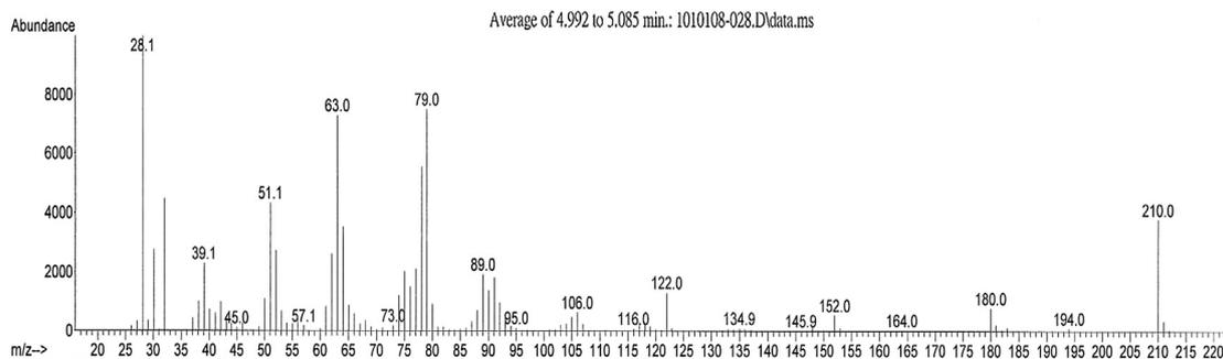
**Fig. 2** – Mass spectrum of formaldehyde-DNP. DNPH = 2,4-dinitrophenylhydrazine.
