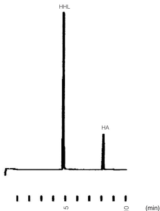
Figure 4. An electropherogram of optimal conditions using the capillary electrophoresis method. (1) standard HHL; (2) standard HA. Experiments were carried out using a fused-silica capillary 65 cm (55 cm to the detector) \times 75 \mu m I.D., 10 mM phosphate buffer at pH 6.0 as the running buffer, an applied voltage of 20 kV, electronic injection time of 2 sec, and a detection wavelength of 228 nm. Sample: a solution of 2.5 mM HA and 2.5 mM HHL in water.
