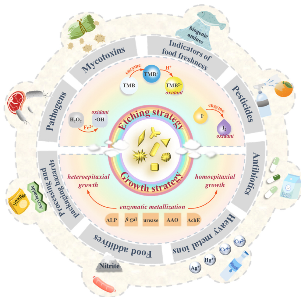
Fig. 1. Overview of the two important strategies for changing the morphology of gold nanomaterials and applications of multicolor colorimetric biosensors based on gold nanomaterials in the field of food hazards detection.
